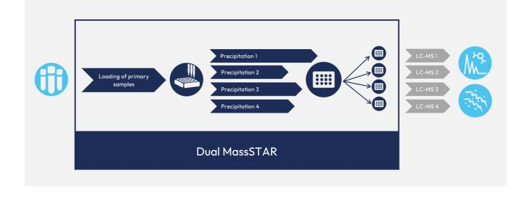
The Dual MassSTAR allows for the combination of analogous protein precipitation workflows for both Drug of Abuse testing and therapeutic drug monitoring. For example, it enables the simultaneous processing of protein
